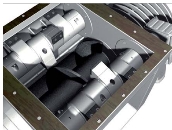
Inside the extruder body with its paddle shafts and cast paddles
