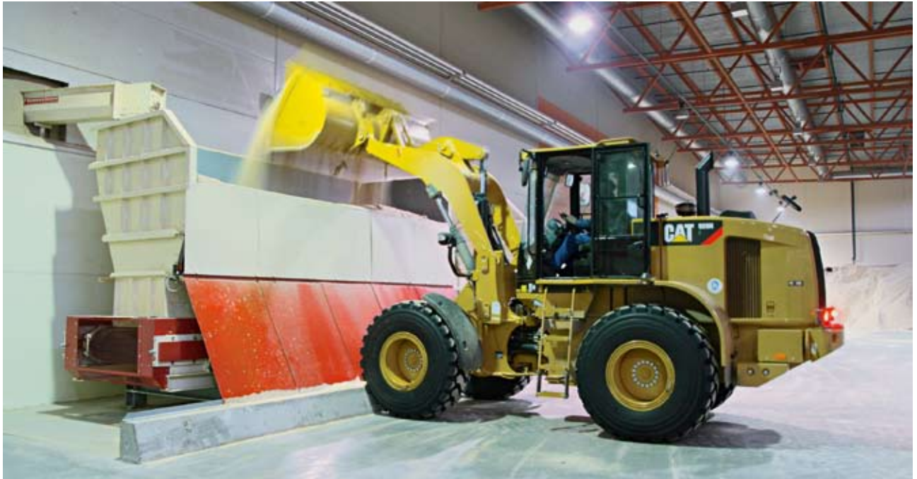
»4 Feeding the sawdust into the rubber-belt box feeder, type BKNG 1206c
