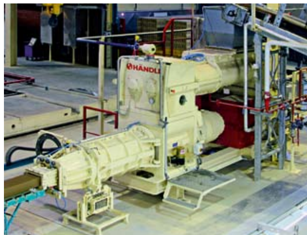
»8 Combined de-airing extrusion unit Futura II comprising a type-MDVG 920f de-airing double-shaft mixer and a type-E56a/50 extruder
