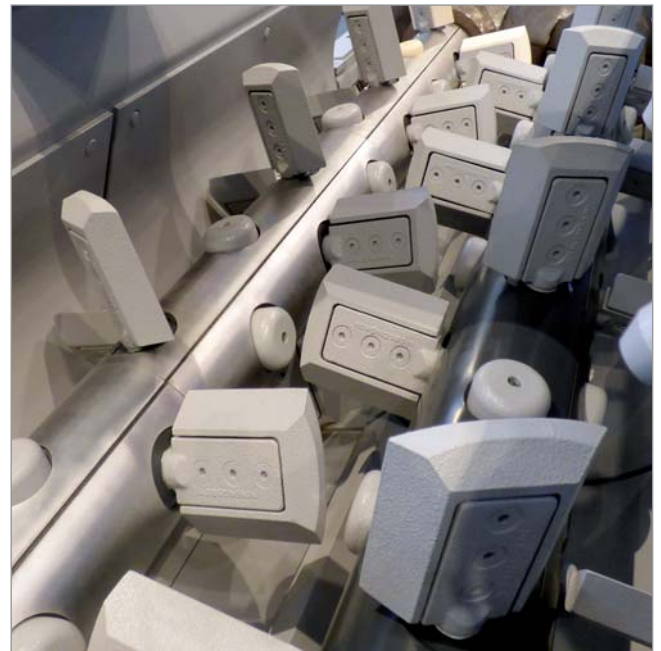
The mixing-zone section of the shafts have protective sleeves. The mixing knives have hard-wearing, replaceable rims as well as hardened protection caps.
